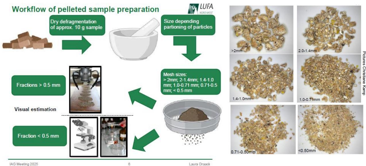
Graph 2: Workflow of pelleted sample preparation and sieve fractions of the PT-sample > 2 mm to <0,5 mm. Pictures taken by Christiane Kamp.
